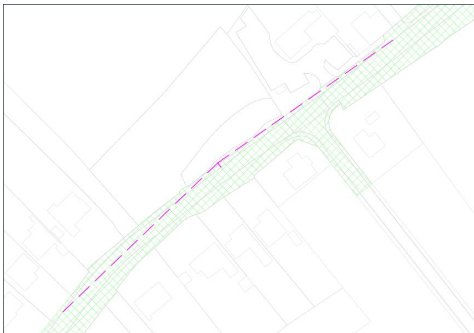
Figure 4-2: 2.4m x 90m Visibility Splays
